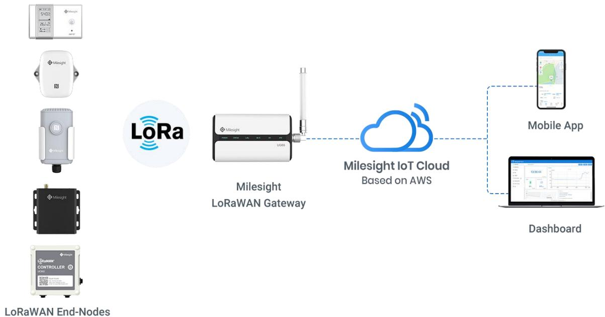
Milesight IoT Cloud provides unparalleled levels of vertical integration with Milesight LoRaWAN® nodes (sensors and controllers). It visualizes field data and enables user to monitor and control remote assets on an intuitive dashboard.
