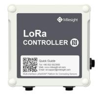
UC50x series is a LoRaWAN® controller used for data acquisition from multiple sensors. It contains different I/O interfaces such as analog inputs, digital inputs, digital outputs, serial ports and so on, which simplify the deployment and replacement of LoRaWAN® networks.
