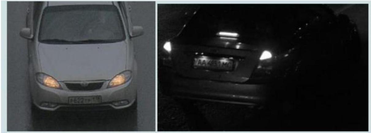
Answer: check the camera already configured to IR night mode. Or confirm the IR light if it is enough, maybe need a separate IR lamp because of the long distance.
