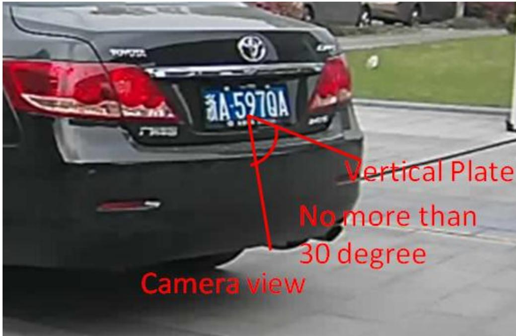
So right now the  $H=5\text{m}$  due to the position of plate is on the lane NO.2 . if we can make the monitor distance( $L$ ) longer like 8 meter, the plate angle will be smaller, but for pixels of plate maybe smaller, because the longer monitor distance, the view of camera will be bigger, so that the pixels of plate reduce.
