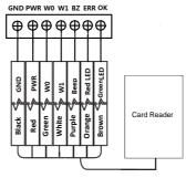
Figure 3-1 Wiring for Wiegand Communication Mode
