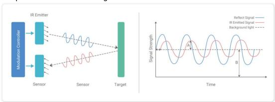
The ToF technology consists of dToF (direct Time of Flight) and iToF (indirect Time of Flight) which are distinguished by different detection methods. For more details about iToF and dToF Technologies, please click: <u>EXPAND</u>:
