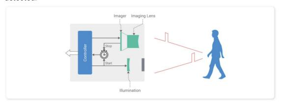
**iToF:** The full name is Indirect Time-of-Flight, indirectly measures the flight time of light by the phase difference. The iToF module emits a modulated infrared signal into the scene, then receives the light signal reflected from the object detected, and calculates the phase difference between the emitted signal and the received signal according to the accumulated charge during the exposure time. It will get the depth information of the target object via the processes.
