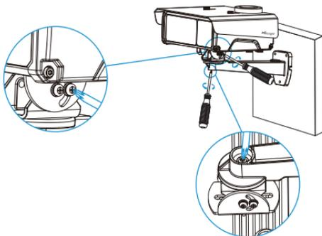
The screws in the bracket section can be adjusted to rotate up and down.
