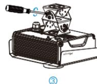
**Step 3:** Place the assembled camera with the bracket onto the gantry. Use screws to secure the bracket to the gantry.
