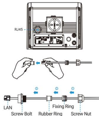
**Step 3:** Insert the Ethernet port into the interface and tighten the waterproof protective cover.
