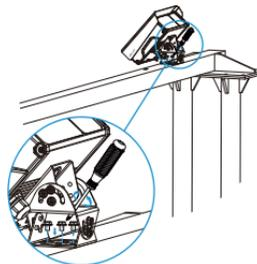
**Step 4:** To adjust the camera angle, loosen the screws indicated on the bracket as shown in the diagram. The bracket can then be rotated for adjustment. Once it is properly adjusted, tighten the screws to secure the bracket in place.
