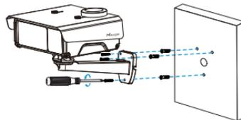
**Step 5:** To adjust the camera angle, loosen the screws indicated on the bracket as shown in the diagram. The bracket can then be rotated for adjustment. Once it is properly adjusted, tighten the screws to secure the bracket in place.
