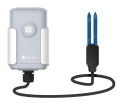
EM500-SMT is designed for measuring soil moisture in harsh environments and transmitting data using LoRaWAN<sup>®</sup> technology. With this low power consumption technology, EM500-SMT can work up to 10 years with 19000 mAh battery. Combining with Milesight LoRaWAN<sup>®</sup> gateway and Milesight IoT Cloud solution, users can manage all sensor data remotely and visually.
