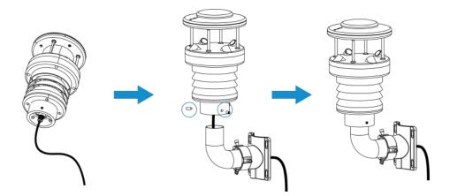
3. Straighten the hose clamps and slide them through the rings in the bracket, wrap the hose clamps around the pole. After that use a screwdriver to tighten the locking mechanism by turning it clockwise. When installing, ensure the arrow on the sensor facing north according to a compass.
