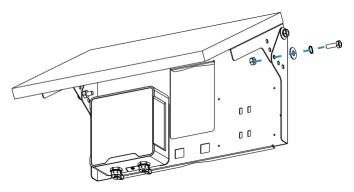
3. Straighten the hose clamps and slide them through the rectangular rings in the solar panel's bracket, wrap the hose clamps around the pole. After that use a screwdriver to tighten the locking mechanism by turning it clockwise.
