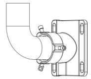
2. Connect one side of sensor cable to WTS Sensor and tighten the cable, pass the cable through the bent pipe and bracket, then connect the pipe to the bottom of sensor and fix both
