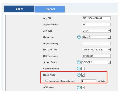
4. After the network connected back, the device will send the lost data from the point in time when the data was lost according to the reporting interval.
