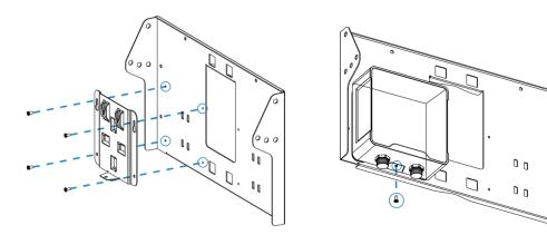
2. Adjust the angle of solar panel brackets (20°,40° or 60° is optional) according to the installation environment, then fix the two sides of bracket with screw kits.
