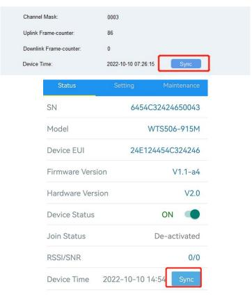
If you set LoRaWAN® version as 1.0.3 or 1.1, the network server will use MAC commands to assign the time to device every time when the sensor joins to network.
