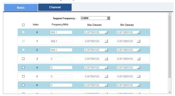
If the frequency is one of CN470/AU915/US915, you can enter the index of the channel that you want to enable in the input box, making them separated by commas.
