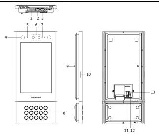
Figure 1-2 Door Station with Keypad Module
