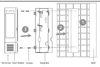
Figure 3-8 Flush Mounting
