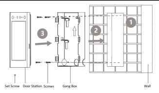
Figure 3-4 Flush Mounting
