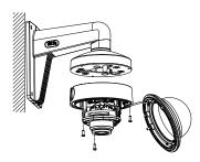
Figure 2-8 Attach the Back Box to the Mount
