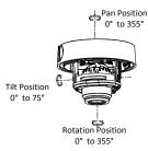
Figure 2-4 3-Axis Adjustment
