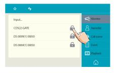
2.Select a Door Station by touching [Unlock] icon to release the corresponding lock.
