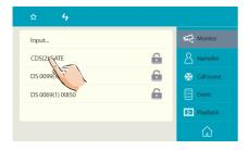
2.Select a Video Door Station by touching it, minitoring is activated immediately. The monitor time is 30 seconds.
