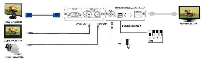
\* 3 outputs: HDMI, VGA, CVBS could be display simultaneously.
