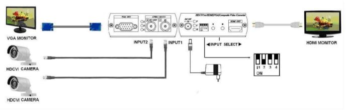
\* Allow two camera inputs with 2 outputs: HDMI, VGA as a switcher.
