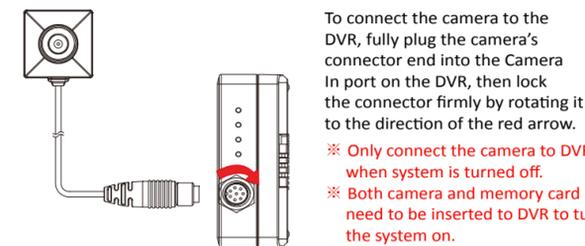
To connect the camera to the DVR, fully plug the camera's connector end into the Camera In port on the DVR, then lock the connector firmly by rotating it to the direction of the red arrow.
