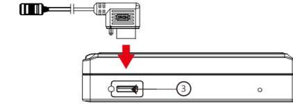
1. Plug in the Controller Cable into the Control port (3).
