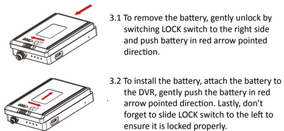
3.1 To remove the battery, gently unlock by switching LOCK switch to the right side and push battery in red arrow pointed direction.
